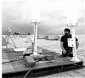
Lightning sensors, such as these, track the electrical charges of lightning strikes. Sensors are important for lightning research, building protection, and forest-fire prevention.
